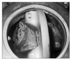
Figure 1 - Valve properly clamped in place.
