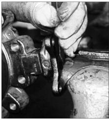
**Figure 2 -** How the upper shaft is removed from the upper disk hub.
